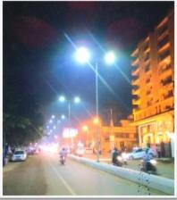
Electrification of LED Lights from Ambedkar Chowk to Employment Office (Main Road) provided with 9 mtr. Octagonal galvanized pole with 90 Watt. LED Light Fittings.
